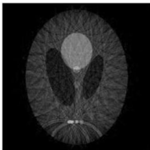
(a) 滤波反投影法结果 (a) Result of FBP method
